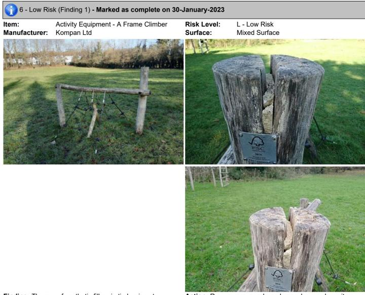
**Finding:** The use of synthetic fillers in timber is not recommended; timber being a natural material will expand and contract as the moisture content changes and the use of fillers can exacerbate the length and depth of these cracks or shakes in the timber. The only treatment that is normally required is the removal of any rough or sharp edges unless the structural integrity of the item is affected.
